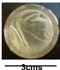
Fig.1. A top view of the feeding chamber used to screen the bacteria through the aphids. Parafilm (a stretchy plastic-similar to cling film) is stretched over a plastic cylinder to form a film over the top. The artificial diet is put on to this film. Another layer of Parafilm is then stretched on top to create a sachet. Aphids are then put inside the cylinder. The aphids move up to the food source and feed as they would from a leaf.
